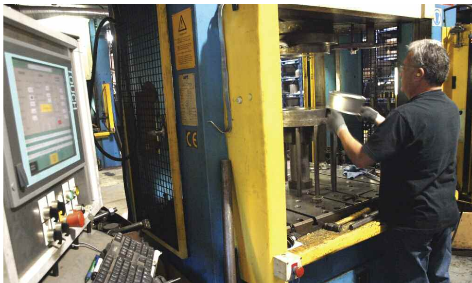
Press operator Dan Tenney tends to the 400-ton hydraulic press at Toledo Metal Spinning, tooled for deep drawing a can. The press resides in a production cell along with plasma-cutting and deburring machines to facilitate one-piece flow.
