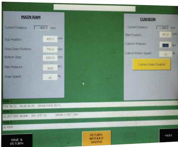
Part of the control-retrofit project included outfitting each hydraulic press with a Siemens Panel PC running Siemens WinCC Flexible application software. Toledo Integrated customized the software to include enhanced operator-friendly screen layouts and diagnostics, to enable on-the-fly parameter adjustments during deep drawing.
